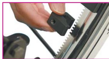
Tilt lock-out stops may be used to limit the tilt range on the low-end, high-end or both.
